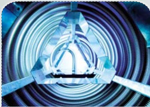
FIGURE 11: Corrugated stainless steel tube (witzenmann.com)
